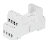
Socket & Clamp (ARSM) 35 mm DIN rail mounting Rating : 6A, 12A, 300V
